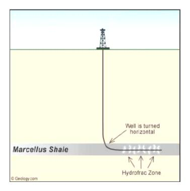
After fracturing some of the frac water "flows back" and must be disposed of. And after the well is put into production, more of this frac wateralong with formation brine water, flows back. This "produced fluid" must also be disposed of.
